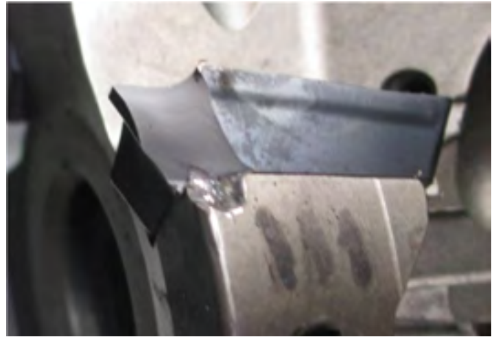
TOOL WEAR OBSERVED ON A CONVENTIONAL MACHINING CENTER AFTER 28 ROUGHING PASSES IN 4140 ALLOY STEEL. REPLENISH COST WAS $924 FOR FOUR NEW INSERTS AND A TOOL BODY REPLACEMENT.
