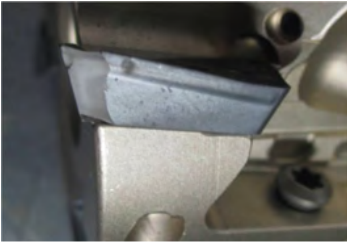
TOOL WEAR OBSERVED ON A HIGH-PERFORMANCE MACHINING CENTER AFTER 38 ROUGHING PASSES IN 4140 ALLOY STEEL. REPLENISH COST WAS $60 FOR FOUR NEW INSERTS.
