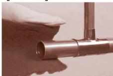
Tools used to ream tube ends include the reaming blade on the tube cutter, half-round or round files (Figure 2), a pocket knife, and a suitable deburring tool (Figure 3). With soft tube, care must be taken not to deform the tube end by applying too much pressure.
