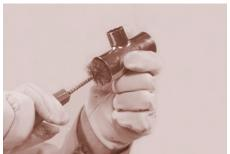
Copper is a relatively soft metal. If too much material is removed from the tube end or fitting cup, a loose fit may result in a poor joint.
