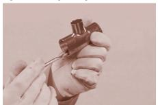
Figure 10. Electric Resistance Soldering Tool
